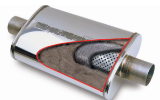
Figure A. Cutout of an absorption (or glasspack) muffler.
